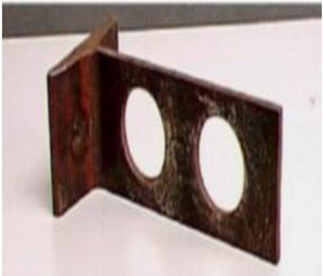
Figure 4. T-RIB shear connector [9].
